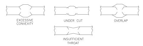
DEFECTIVE BUTT WELD PROFILES FIG.28
