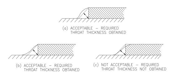
FILLET WELD EQUAL TO THE SIZE OF PLATE OR SECTION FIG.-16
