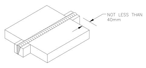
BUTT WELDED JOINT WITH RUN-ON AND RUN-OFF PLATES
