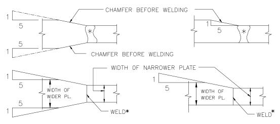
TRANSITION BY CHAMFERING THICKER OR WIDER PART FIG. -3
