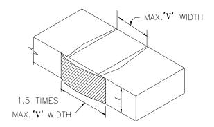
BUTT WELD END REINFORCEMENT FIG. -9
